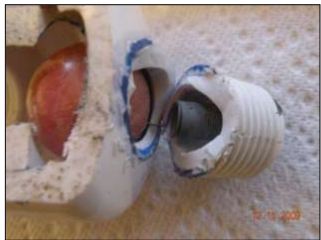
(closeup: negligible buildup after 4 years)
