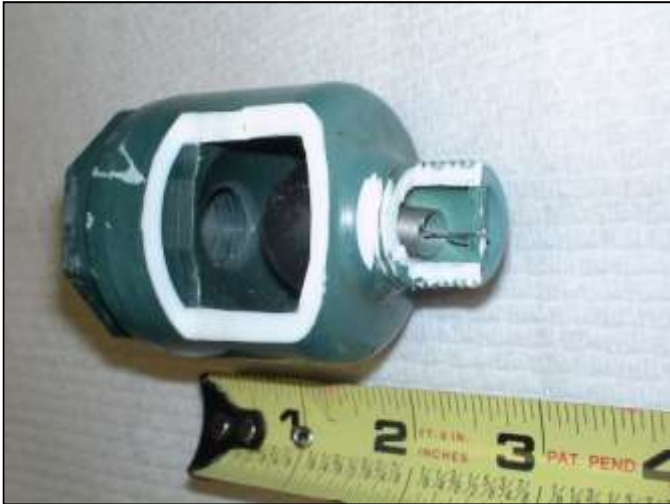
(Negligible deposits at the bottom of the unit)
