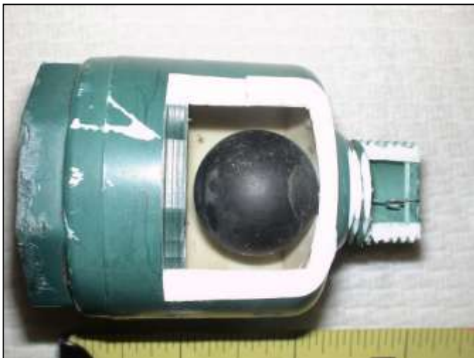
(No debris buildup at the inner-top of the unit)
